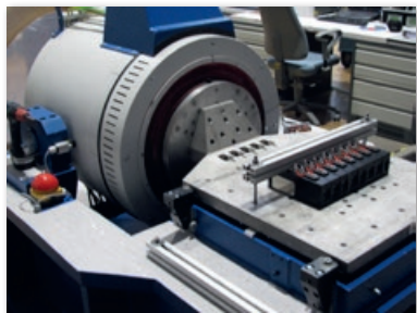
Horizontal tests of electronic equipment
